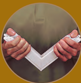
Pinch fusion-welded strength
