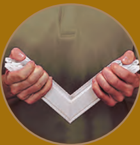
Pinch fusion-welded strength
